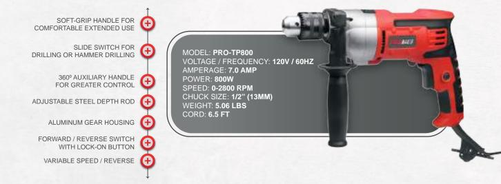
INCLUDES: 1/2" (13mm) Hammer Drill. Side handle. Depth Rod. Key Chuck.
