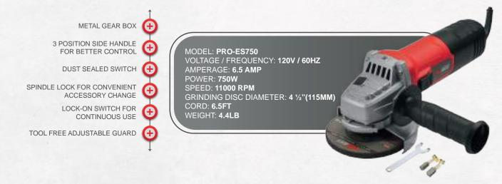
INCLUDES: Angle Grinder, Side Handle, Wrench, 1 Abrasive Wheel, 2 Carbon Brushes.
