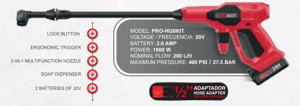
**INCLUDE:** Wireless pressure gun, 2 batteries 20V, battery charger, 2 connection adapters, pressure hose, 5-in-1 multifunction adapter, cleaning wire for nozzle, storage bag, soap tank, pressure extension lance.
